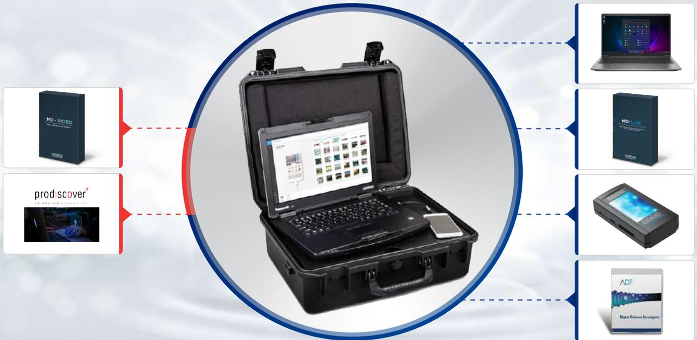
The US-Forensic Field Kit consists of a high-performing forensic laptop built for law enforcement investigators to handle forensic triage, acquisition, and analysis challenges on-field for Forensic Data Recovery from Evidence devices.
